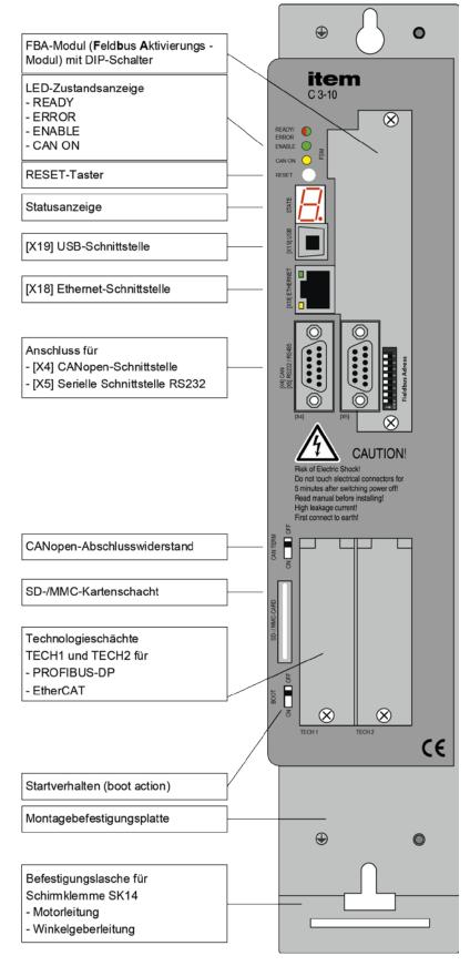
Figure 9: item Servo Positioning Controller C 3-10: front view
