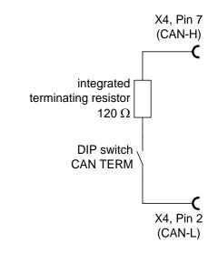
Figure 26: Integrated CAN terminating resistor
