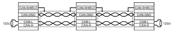
Figure 25: CAN bus cabling example
