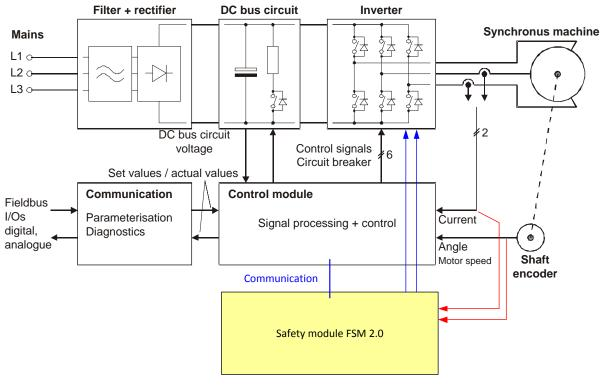
Figure 6: Schematic representation of the integrated safety technology
