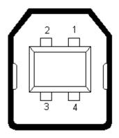
Figure 28: Pin assignment USB interface [X19], front view
