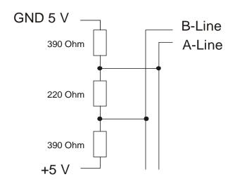
Figure 31: PROFIBUS-DP interface: connection with external terminating resistors
