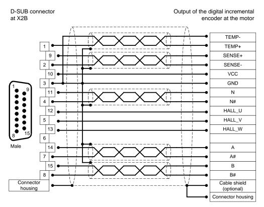
Figure 22: Pin assignment: digital incremental encoder - option [X2B]
