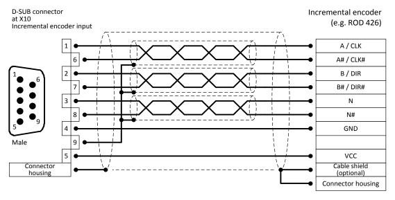
Figure 23: Pin assignment [X10]: incremental encoder input
