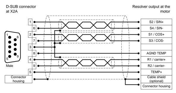
Figure 19: Pin assignment: resolver connector [X2A]
