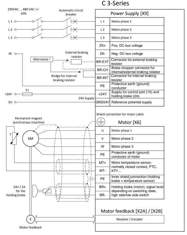
Figure 13: Connection to the power supply and motor
