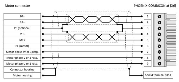
Figure 16: Motor connector [X6]
